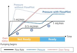
**FlowPilot** (Patent Pending) The pump controls the flow rate according to oven temparature. The flow rate is gradually increased up to half of the set value.(①) The flow rate is kept constant until the oven is ready.(②) The flow rate is gradually increased up to the set value.(③)
