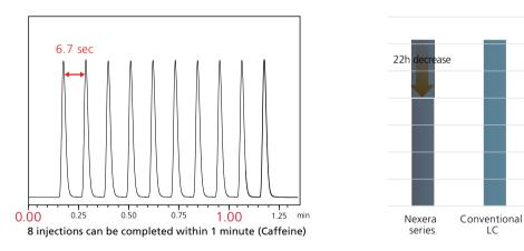
Pharmacokinetic analysis requires not only speed but also high reliability at low concentrations. With its ultra-fast injection and ultra-low carryover, the SIL-40 autosampler delivers high reproducibility and reliability, even during an ultra-fast 30-second analysis.
